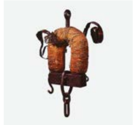
Joseph Henry's electromechanical relay
