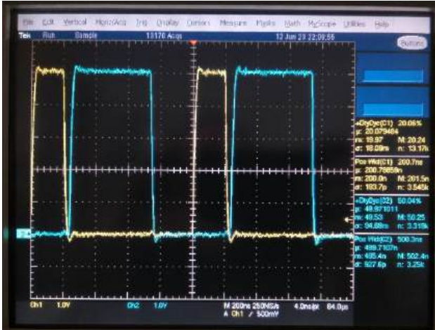
Figure 19: Extension of the 200 ns pulse with monoflop to 500 ns.
