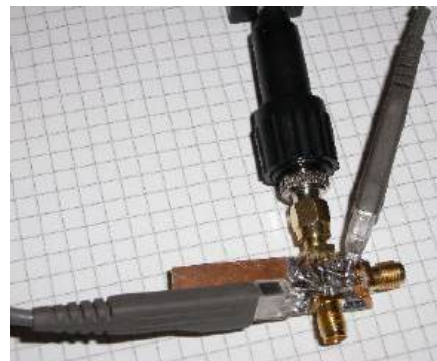
Figure 8: Left: schematic setup for measuring the phase progression of the inductors; Right: Lab setup of the measuring adapter.
