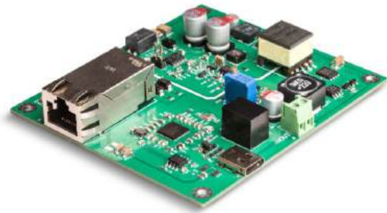
Figure 9: GB Ethernet USB adapter with PoE.
