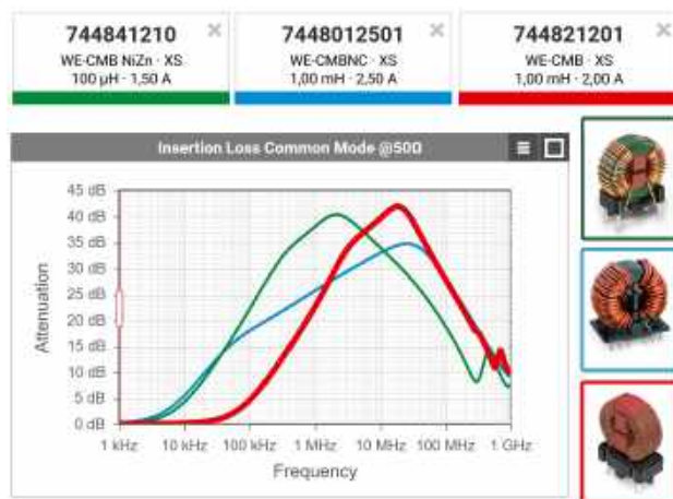
Figure 40: Insertion loss (common mode) measured for three common mode chokes with different core materials from 1 kHz to 1 GHz.
