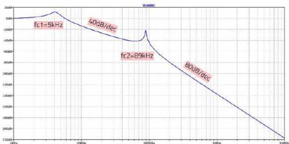
Figure 48: The two-stage filter attenuation behavior.
